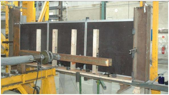
Figure 7 : Bending test rig
