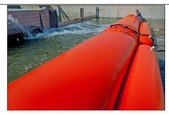
Fig. 1: Double tube flood protection system OPTIMAL in the testing facility of the TUHH in April 2011<sup>1</sup>
