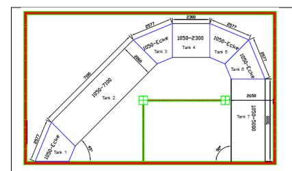
Fig. 4: Product configuration according to the FM Approval in the testing facility of the TUHH in Hamburg-Wilhelmsburg<sup>11</sup>
