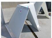
Hexagonal Aluminium comb panel "ALUCORE 15<sup>1</sup>" + Aluminium coating
