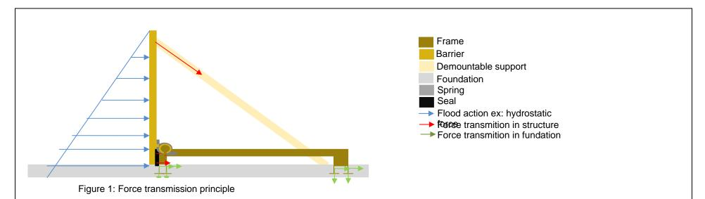
The opening mechanism is a flap system. As the weight of the used steel material is important, springs at the rotation axis enable an easier mobilisation process by hand. The spring effect can be adjusted thanks to a mechanism which varies the energy transmitted by the spring.
