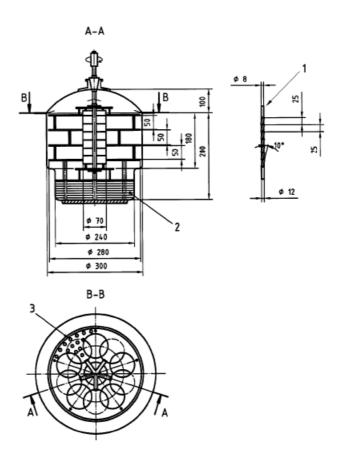
Figure 22: Evaporation atmosphere (BS EN 1931) 1 side view of the propeller with blades. 2 saturated salt solution with remaining solid at the bottom. 3 125 holes  $\Phi$  8 per plate
