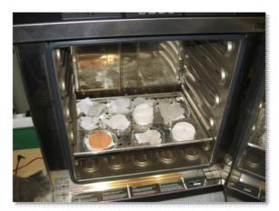
Figure 18: Building material test samples in the drying oven to determine their oven-dry mass.
