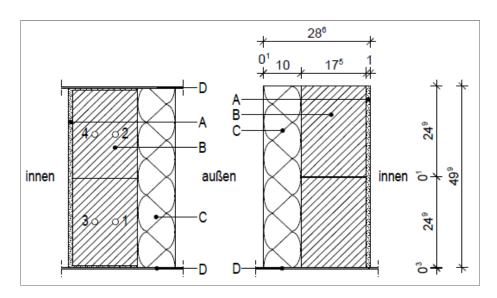
Fig. 15: Composite wall construction; single shell wall of light (aerated) concrete blocks with thermal insulation composite system.
