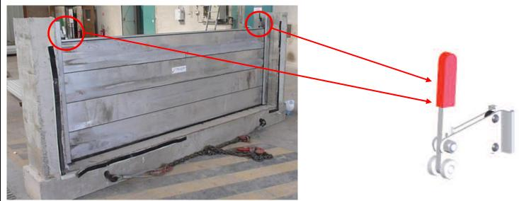
Figure 1: Barrier n°4 elements stacked between columns
