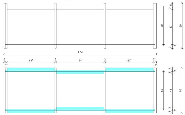
Fig. 20: Schematic of the water tank used for testing. Top: plan. Bottom: side elevation without frame.
