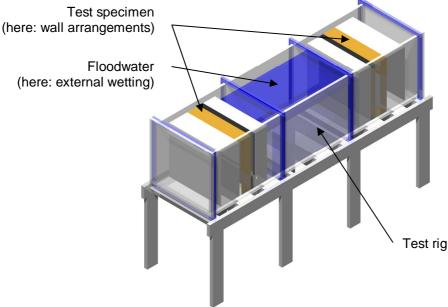
Figure 12: Top: Schematic plan of the water tank used for testing. Bottom: Oblique view of the water tank with two test specimen.
