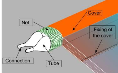
Fig. 1: Modildeich MD93-2 installed at the water basin of the TUHH
