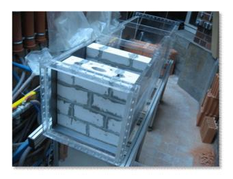
Figure 16: Water tank with two wall test arrangements that are under construction in-situ. In front: the double shell masonry of sand-lime bricks with heat insulation and air gap. In the background: the single shell masonry of hollow bricks with external heat insulation and ventilated curtain façade.
