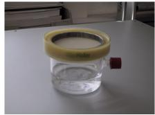
Figure 7: Water vapor permeability
