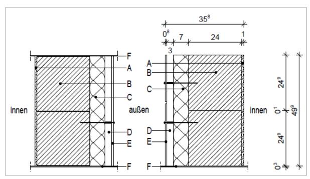
Fig. 11: Composite wall construction; single shell masonry of hollow bricks with external heat insulation and ventilated curtain wall;
