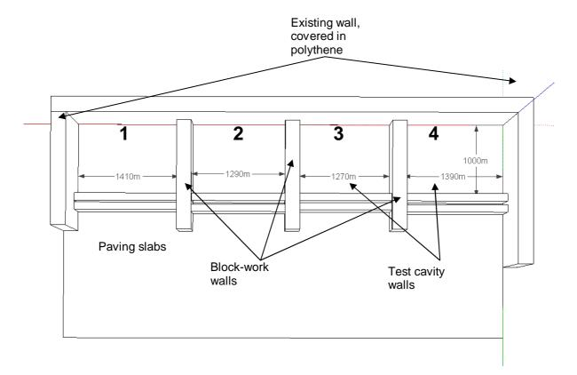
Figure 11: Plan view of the test tanks
