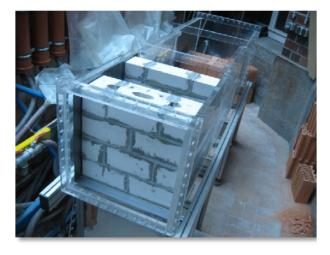
Fig. 24: Water tank with two wall test arrangements that are under construction in-situ. In front: the double shell masonry of sand-lime bricks with heat insulation and air gap. In the background: the single shell masonry of hollow bricks with external heat insulation and ventilated curtain facade.
