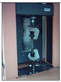
Figure 18 Lloyd Instruments. Testing facilities of mechanical properties test for rectangular speciments(3-5 mm and 20mm ±10%)
