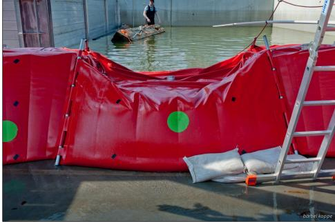
Fig. 8: Straight product configuration of the system DADLER in the testing facility of the TUHH in Hamburg-Wilhelmsburg<sup>14</sup>
