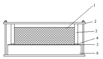
Figure 19. Schematic diagram of apparatus .EOTA TR 012 1 – water (anti-evaporation balls not shown); 2 – clamp; 3 –reservoir; 4 – sealant; 5 – liquid waterproofing system; 6 – substrate.
