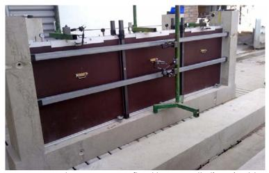
Figure 2: Hydrostatic test on flood barrier Collad'eau (width 3m)
