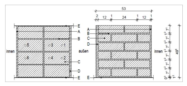
Fig. 13: Composite wall construction; single shell masonry of traditional solid bricks during construction
