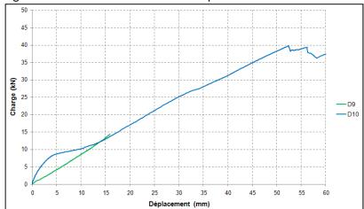
Figure 14: load-deformation curve on panel P3
