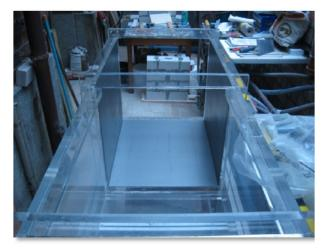
Fig. 21: Steel plates for the lateral connection
