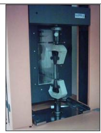
Figure 2 Lloyd Instruments. Testing facilities of mechanical properties test for rectangular speciments(3-5 mm and 20mm ±10%)
