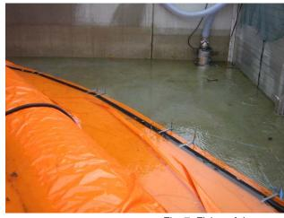
Fig. 5: Configuration of the Mobildeich using steel dowels
