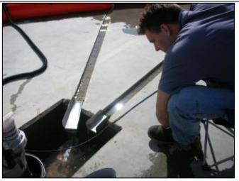
Figure 10: Pump sump for leakage measurement<sup>3 oben3</sup>
