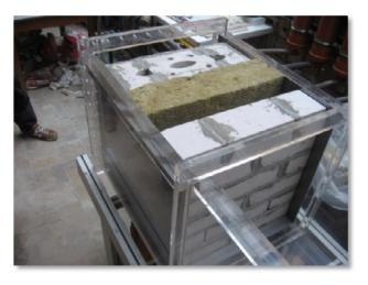
Fig. 8: Composite wall construction; double shell masonry of sand-lime bricks with heat insulation.
