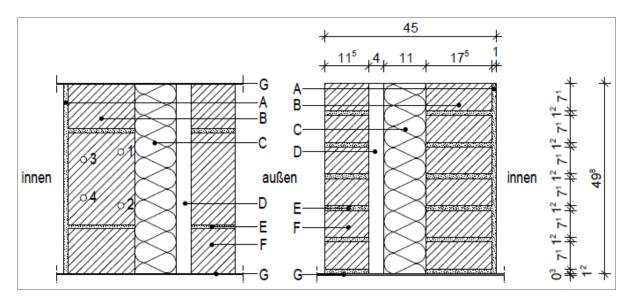
Fig. 9: Composite wall construction; double shell masonry of sand-lime bricks with heat insulation;
