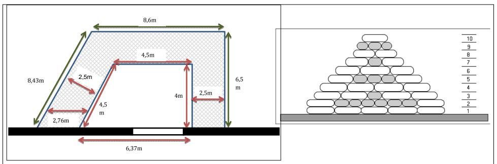
Fig. 4: Product configuration according to the FM Approval in the testing facility of the TUHH in Hamburg-Wilhelmsburg<sup>22</sup>
