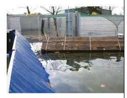
Figure 5 : Hydrodynamic load / current load executed perpendicular to the barriers
