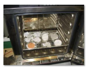
Fig. 26: Building material test samples in the drying oven to determine their oven-dry mass.
