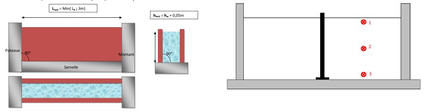
Figure 2: Water tightness test rig and positioning of deflection measurements points
