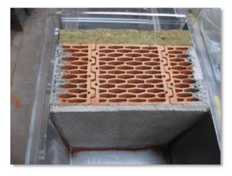
Fig. 10: Composite wall construction; single shell masonry of hollow bricks with external heat insulation and ventilated curtain wall; the curtain façade board is not yet mounted here.
