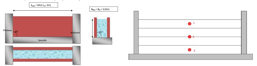
Figure 3: Water tightness test rig and positioning of deflection measurements points
