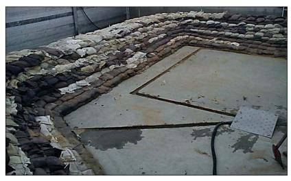
Fig. 6: Filled sandbags on pallets and built sandbag dam according to FM Approval in the testing facility of the TUHH in Hamburg-Wilhelmsburg<sup>22</sup>
