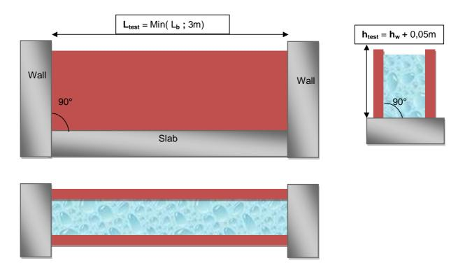
Figure 9: CSTB hydrostatic test facility
