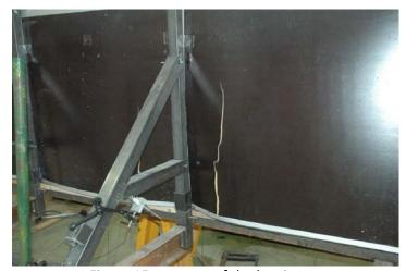
Figure 15 : rupture of the barrier
