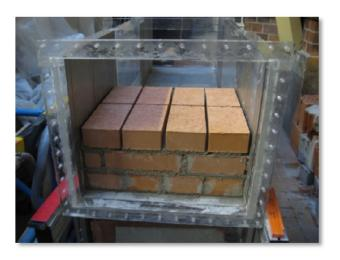
Fig. 12: Composite wall construction; single shell masonry of traditional solid bricks during the construction phase.
