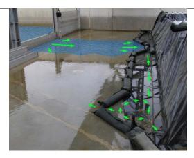
Figure 15: Product state after current load perpendicular to the barrier at low water depth
