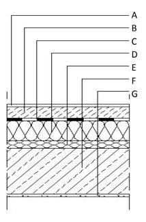
Fig. 19: Cross-section of the tested concrete floor; et), (B) cement screed, (C) Separation layer (PE-film), (D) heat in
