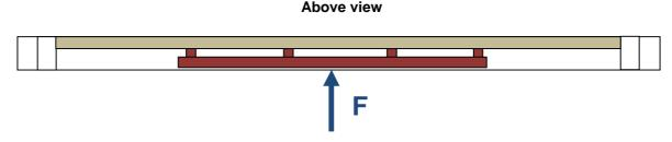
Figure 10: CSTB bending test facility
