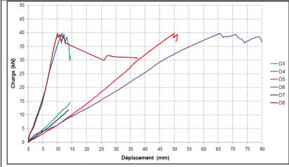
Figure 13 : load-deformation curve on panel P2
