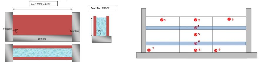
Figure 6: Water tightness test rig and positioning of deflection measurements points
