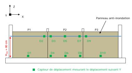
Figure 12: disposition of the measurement key points
