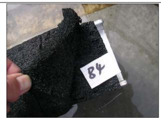
Fig. 9: Cracked ground seal at the end of the destructive testing<sup>36</sup> **Suggestion for improvement**
