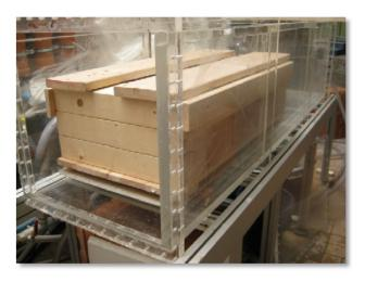
Fig. 16: Suspended timber floor; test arrangement consisting of structural joists, heat and sound insulation, plasterboard ceiling, and covering floor
