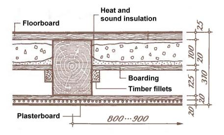
Fig. 17: Cross-section of the timber floor
