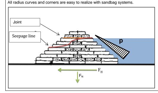
Fig. 1: Possible seepage line in a sandbag dam<sup>17</sup>
