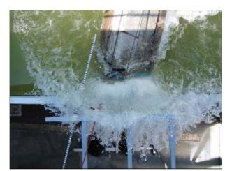
Fig. 6: Impact of flotsam at the IBS Mobile Wall System<sup>36</sup>
