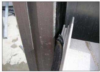
Fig. 7: Loose seals at the end of the destructive testing<sup>36</sup>
