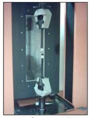
Figure 17 Lloyd Instruments . Test facility of adhesion test for rectangular speciments(wide:25mm ± 5% and long: 100mm±5%) Velocity of test: 3 mm min-1
