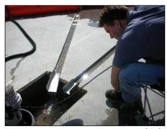
Figure 10: Pump sump for leakage measurement<sup>3 oben3</sup>
