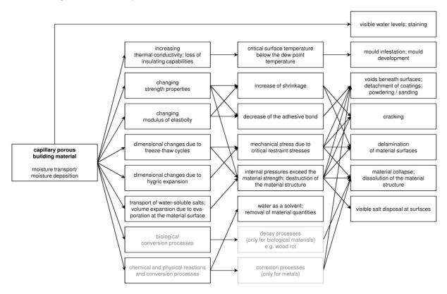
Fig. 1: Scheme of potential flood damage processes.
