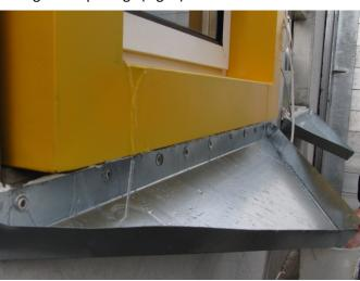
Fig. 4: Aluminium plates to measure the leakage
